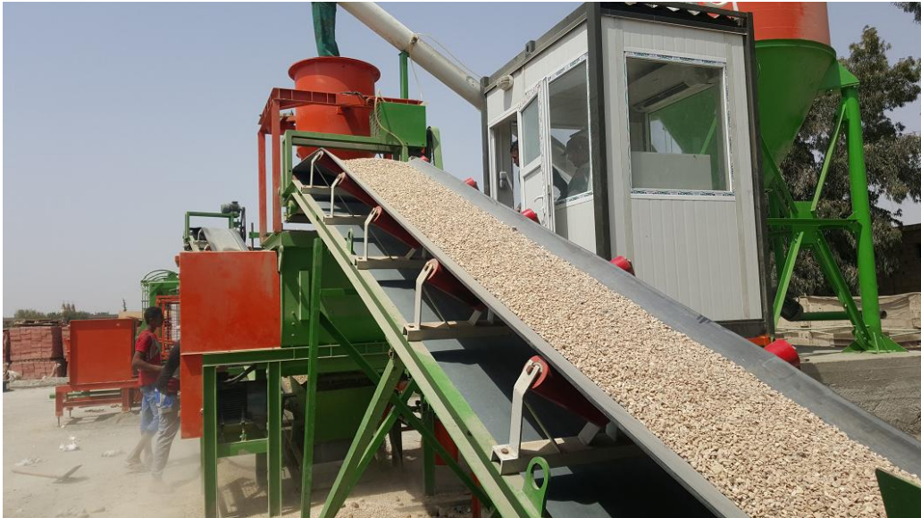
View of Sand Conveyor Belt
